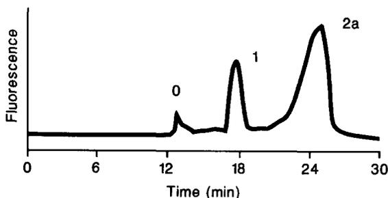
**Figure 1b** Typical molecular exclusion (TSK) chromatogram of human holo-RBP. Chromatogram is of 25  $\mu\text{L}$  of 1:3 diluted human plasma. HPLC method is as described in text.
