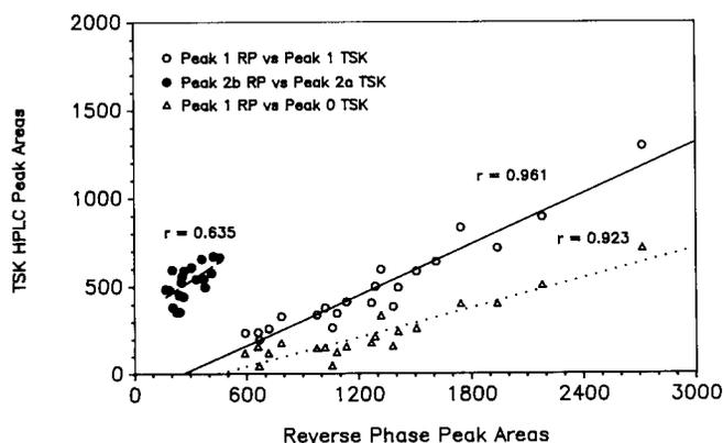
**Figure 3** Correlation of peak areas determined by molecular exclusion HPLC with peak areas determined by reverse phase. Methods as described in text.
